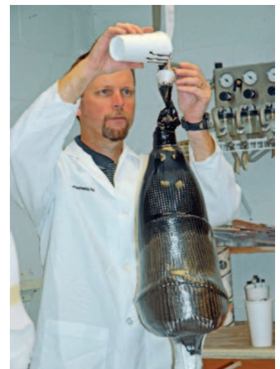
Adding catalyst-pigment mixture to activate socket lamination.
